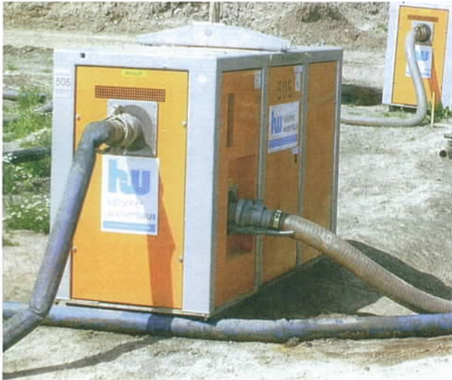
Figure 5. Piston pump connected to a drainage system.
