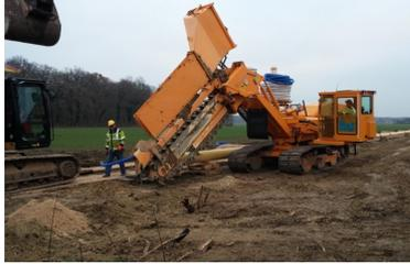
Figure 3: The GIGANT 3600 digs trenches up to 4500 mm deep (minimum depth: 1500 mm), covering the requirements of 80 % of customer enquiries.
